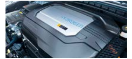
The fuel cell works by passing hydrogen and air through a fuel cell stack.
