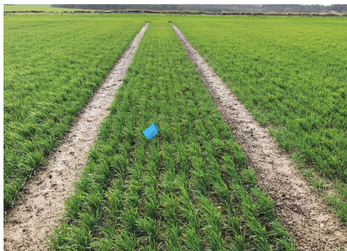
Pegging out – small flags mark where the source (red flag) and receiver (blue flag) points are to be.
