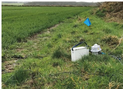
Receivers – record sound waves returning from the earth below.
