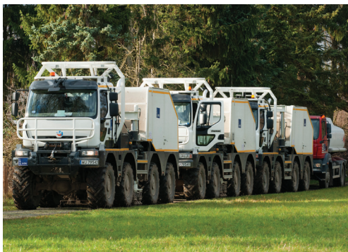
Vibroseis trucks – create the downward energy by vibrating a steel plate on the ground.
