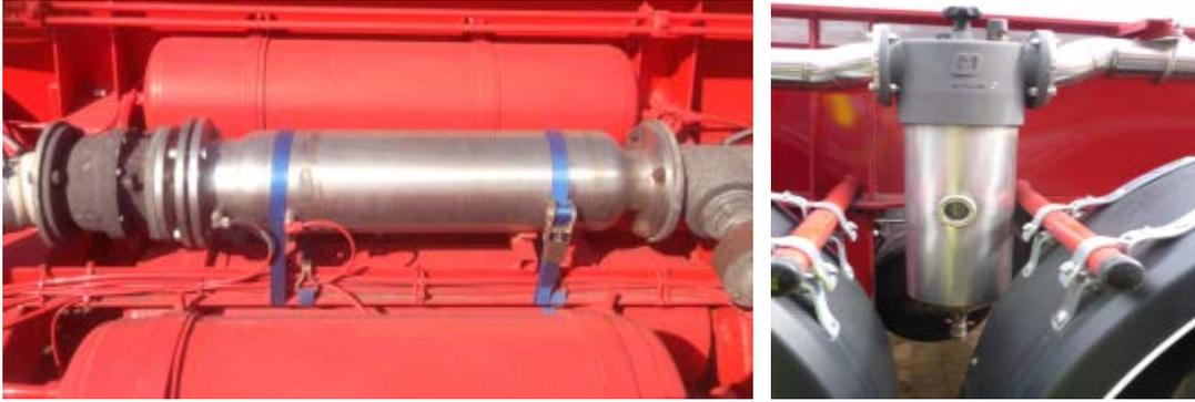
**Compressed Air Filter, typically 5micron in size, to the rotary valve.**
