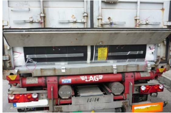
11.5.9 Remove the tundish, clean thoroughly using the compressed air line. When clean, attach the tundish to the discharge opening at the rear of the container. Ensure the retaining bolts are fully extended and fixed in place.
