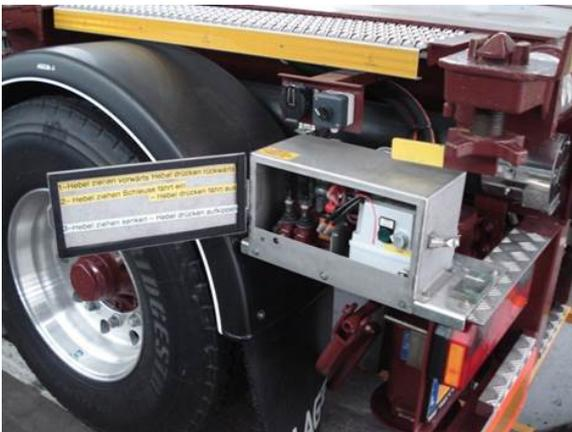
Compressor and Rotary valve - side operation
