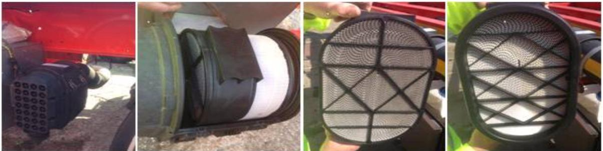
**Air intake filtration system for SDU chassis.**
