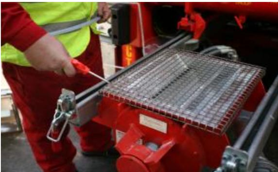
Rotary Valve Cleaning with safety grid in place.
