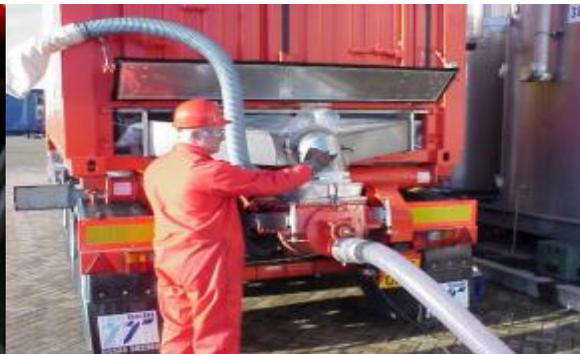
Rotary valve set up for "discharge Operations".
