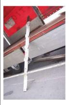
**Curtain sider or tautliner** (trailers without side boards and with tarpaulins which slide along the roof structure like a curtain)
