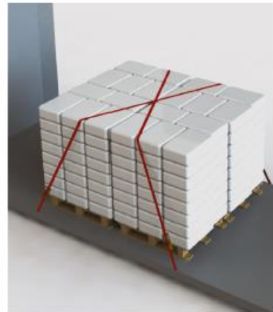
4 pallets with cross lashing
