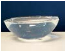
First production of virgin polystyrene from only depolymerised material
