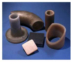
FRP parts fabricated using various fabrication processes.
