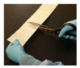
Lay out fiberglass mat strips on the work surface and cut each strip to the appropriate length
