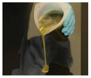
After thoroughly mixing in the initiator, pour the resin onto the release film
