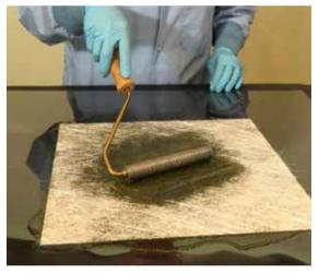
Roll with a serrated roller
