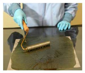
Apply veil layer and roll with a serrated roller
