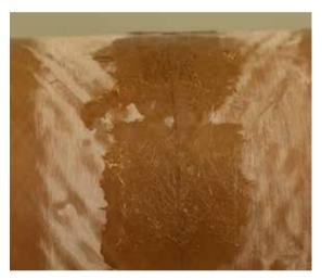
Curing or hardening in a matter of minutes, the "patches" or "tabs" secure the pipe sections in the proper alignment
