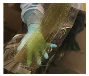
Pick up the completed weld strip
