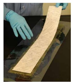
Place the next-widest strip of fiberglass onto the first with one end of the second strip starting approximately 3 cm (1 in) in from the end of the first strip
