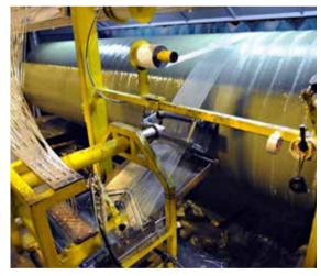
Filament winding process.
