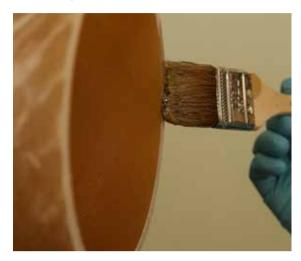
Coat roughened end edges of pipe with a small amount of initiated resin
