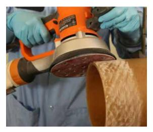
Roughen the outside surfaces with a sander approximately 3 cm (1 in) farther in from the ends than the finished weld surface; where inside welds are possible, interior surfaces should be sanded prior to assembly
