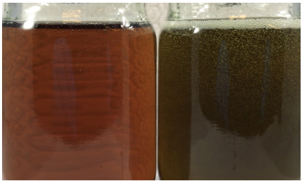
Figure 2: Comparison of foaming in promoted and initiated Derakane™ Signia™ 411 (left) and Derakane™ Momentum™ 411 (right) resin 90 seconds after initiation.
