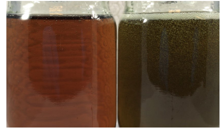
Figure 2: Comparison of foaming in promoted and initiated Derakane™ Signia™ 411 (left) and Derakane™ Momentum™ 411 (right) resin 90 seconds after initiation.
