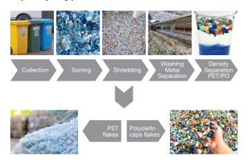
INEOS O&P Europe offers three New Recycl-IN HDPE Hybrids with 50% PCR based on caps from PET bottles, tailored made for non-food caps applications & technical injection applications:
