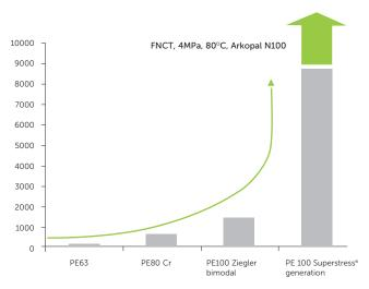
Slow Crack Growth Resistance of ELTEX® Superstress® resins exceed several years under FNCT (80°C, 4MPa) exhibiting outstanding resistance against overall slow crack growth mechanism.
