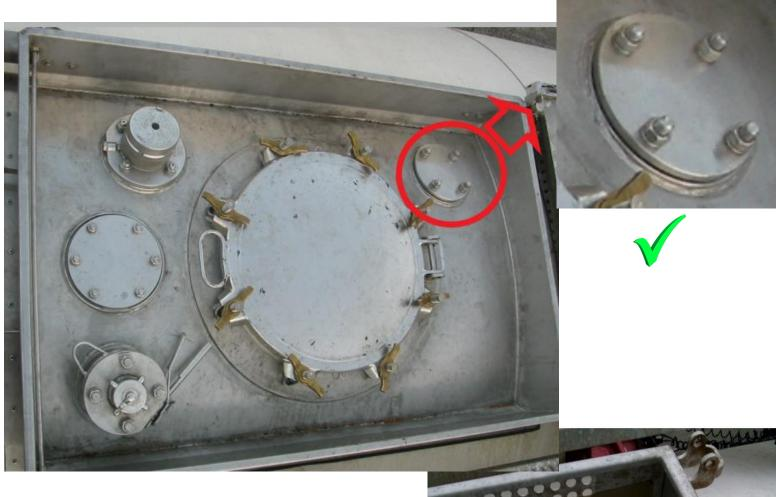
A sunken Flange is not recommend this could lead to a rejection (the fitting piece has a higher pressure class and is a little bit broader then the flange). Optimal will be a flange with a raised position as shown in the picture on the top.
