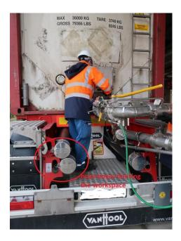
Maximum allowed distance from the end of the chassis (outside) to the end of installed fitting piece is 50cm.
