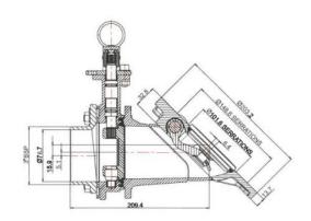
Experience shows that a long design of the Bottom valve is recommend, like the Fort Vale example with a length of approx. 209mm (close to the end of the cabinet). The dimensions of the cabinet should be approx. height 398mm, wide 602mm and maximum depth of 443mm to ensure a maximum workspace.
