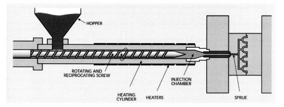
Premature gate freeze-off, stopping the flow of compensatory material to the cavity is the common problem encountered. This generally requires that temperatures be increased and injection pressure and hold times be adjusted to prevent sinks and warpage.
