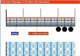
These trailers require at least two transversal straps per row of UNT14 portable tanks.
