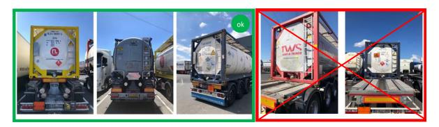
All vehicles for bulk product transport shall be equipped with 3 independent closures in series for bottom filling or discharge openings. This includes an internal valve (bottom / foot), an external valve and a final closing device.
