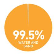
FRACKING FLUID IS 99.5% WATER AND SAND. THE OTHER 0.5% IS MADE UP OF BASIC ADDITIVES.
