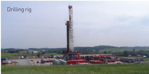
**Drilling equipment:** A rig capable of drilling to the target depth would have a maximum operating height of 60 metres. The rig is modularised and will be delivered by lorry and assembled on site.
