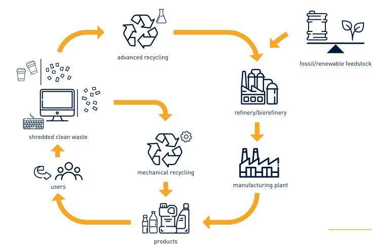
where the plastic waste recovered is physically processed into reusable form; and advanced recycling, in which the waste plastic is either broken down chemically into its constituent parts for repolymerisation into new polymer, or recovered in pure form after dissolution in a solvent.
