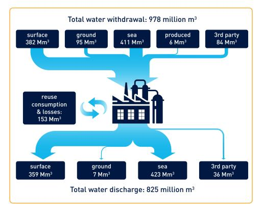
Best available technologies, such as closed-loop water systems and procedures to reuse process water or condensates onsite or at neighbouring production plants, are standard practice at INEOS sites.
