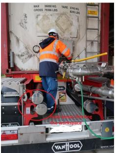
Maximum allowed distance from the end of the chassis (outside) to the end of installed fitting piece is 50cm.
