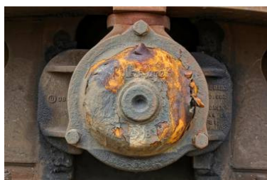
Rust formation due to overheating
