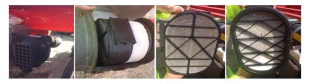
Air intake filtration system for SDU chassis.
