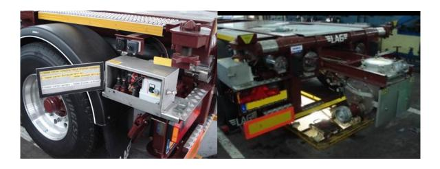
Compressor and Rotary valve - side operation
