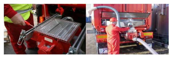
Rotary Valve Cleaning with safety grid in place.
