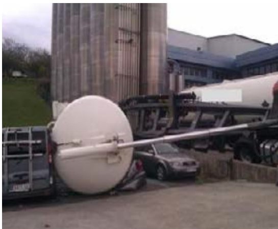
Trailer fell on parked cars during tipping
