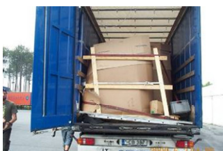
Octabin collapsed resulting in spillage
