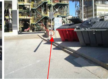
Barrier in half open position. Open end almost not visible to upcoming traffic
