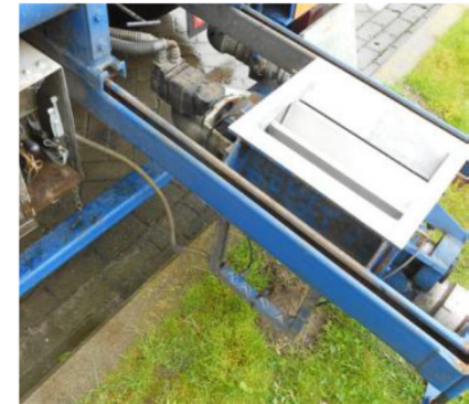
Rotary valve without safety grid
