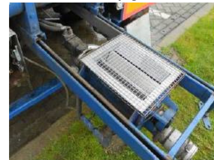
Rotary valve with safety grid
