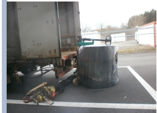
Pallet with FFS coils and hand pallet truck
