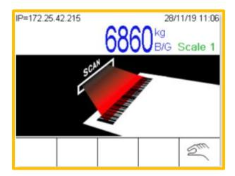
The driver has to scan the ticket with the barcode he received at the kiosk. This to identify the right Ineos reference. It's also possible to type the reference manually by clicking the hand at the right bottom.
