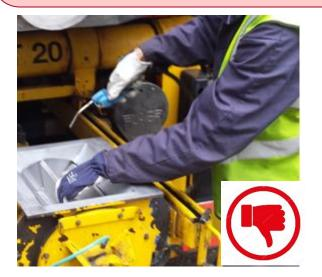
When cleaning the rotary valve, do NOT insert your hand inside the valve.
