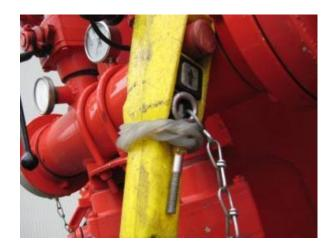
Overriding the dead man system of the operating mechanism to raise the silo!
