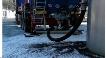
It is paramount to use a restraint system like safety clamps on all connections before discharge can start.
