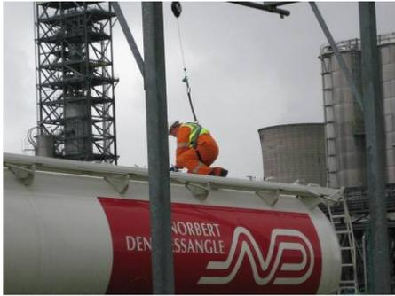
NOK: Handrail truck can not be put up because access step is resting on it
