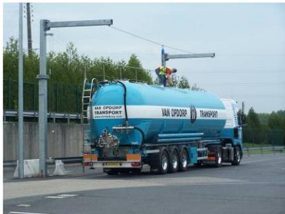
OK: Simple life line system: cable between two poles, handrail truck up
